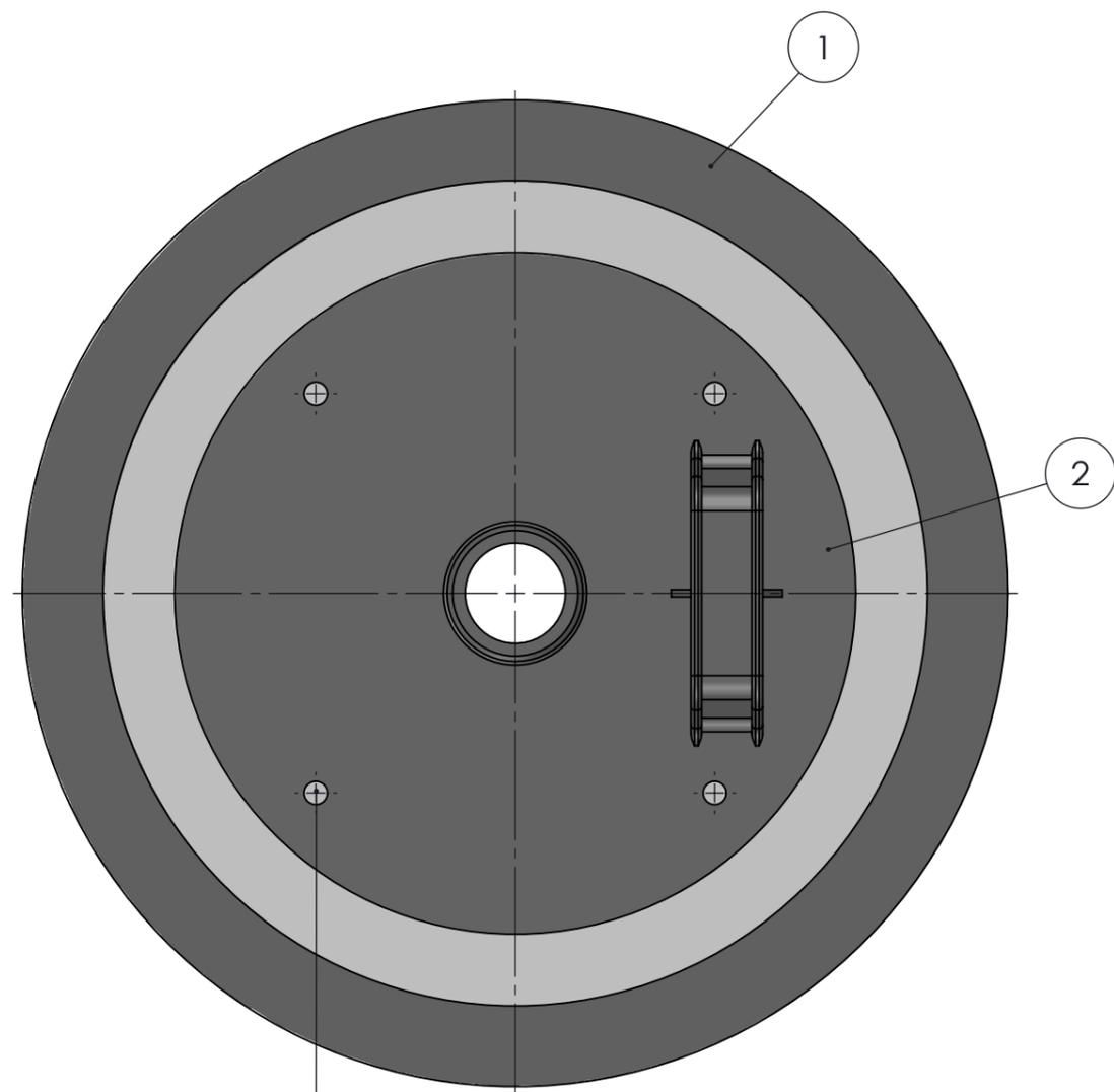
ASSEMBLARE CON N.4 RIVETTI
