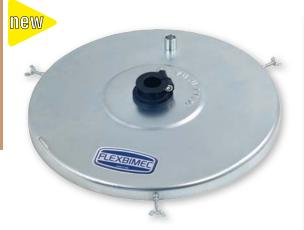
Metal drum cover, available in different dimensions to suit to the various types of grease drums, including butterfly screws for the fixation of the cover on the drum as well as bung adapter for the fixation of the pump in vertical position.
