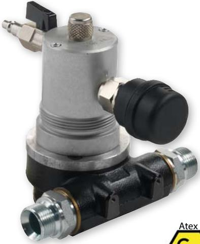
Pneumatic, selfpriming rotary vane pump for the transfer of petrol, with body in cast iron with anticorrosive coating and plastic rotor. On demand the pump can be supplied with an earth cable to enable an electrostatic discharge.
