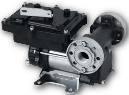
Electric, selfpriming 12 VDC – rotary vane pump (on demand also available in 230 VAC) for the transfer of petrol, with painted body in cast iron with anticorrosive coating, anti-noise filter (electromagnetic compatibility EMC), thermal protection, non-return valve, pressure relief valve, built-in bypass valve.
