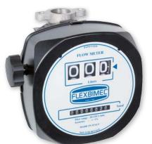
Mechanical nutating – disk flow meter for petrol, kerosene and diesel, with 3 – digits partial meter (max. 999 l; resettable to zero) and 8 – digits totalizer (non resettable). The meter can easily be calibrated and it can also be used for gravity applications. The upper part can be rotated so that different flow directions are possible.
