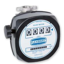
Mechanical nutating – disk flow meter for petrol, kerosene and diesel, with 4 – digits partial meter (max. 9999 l; resettable to zero) and 8 – digits totalizer (non resettable). The meter can easily be calibrated and it can also be used for gravity applications. The upper part can be rotated so that different flow directions are possible.
