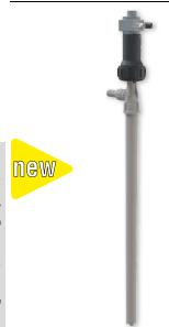
Body and suction tube in PVDF, shaft in HASTELLOY, gaskets in Viton®.
