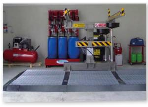
Vehicle ramp in painted steel for vehicle placement, with working platform composed of spill containment safety floor for the collection of eventually leaking fluids.
