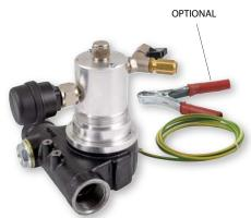
Pneumatic, selfpriming rotary vane pump for the transfer of petrol, with body in cast iron with anticorrosive coating and plastic rotor. On demand the pump can be supplied with an earth cable to enable an electrostatic discharge.
